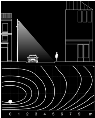
ST1 / Type II Short Street Optic for intense vehicle traffic, urban and suburban areas
